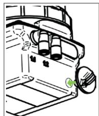
1. Turn the activation and programming key to the OPEN position and remove it from the housing of LUB-B.
