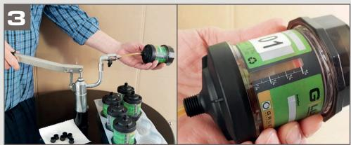
While filling G-LUBE, rotate the device around its own axis to to allow the lubricant to spread evenly. The number of strokes depend on the lubricant and the size of the unit. As soon as you sense a slight backpressure the device is filled completely.
