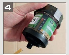
Remove the hose carefully and clean the outlet. Now the device may be screwed on to the lubrication point.
