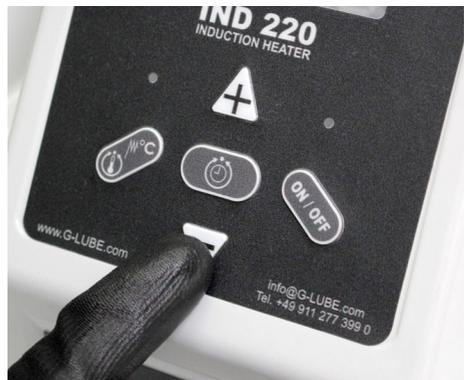
Fig. 15, 16: Ajustar a temperatura
