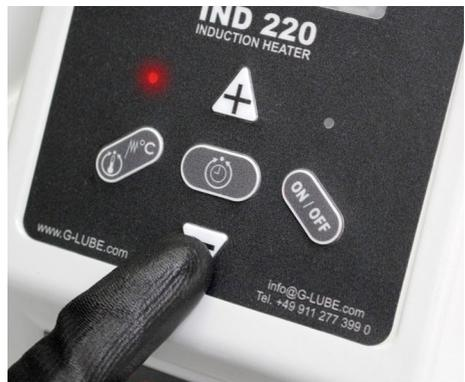
Fig. 10, 11: Ajustar a temperatura
