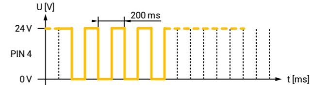
Information about the status of LUB-V and about the past motor run can be evaluated via an evaluation of the number of edge changes of the output signal. For the evaluation of the edge changes, the rising edge must always be counted. The counted number of edge changes corresponds to a one-to-one state of LUB-V.
