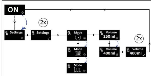
If you would like to change the operating mode, select the Settings menu and move the activation and programming key back to the action area when Mode is displayed.
