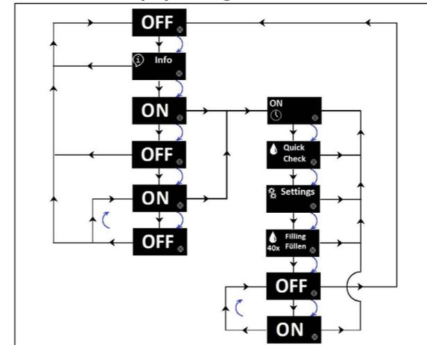
The graphic above illustrates the unchangeable basic flowchart of the LUB-V menu navigation as well as the options for branching to submenus.
