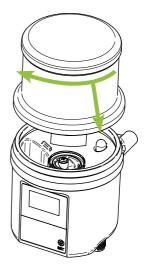
(1) The end position should be reached after two full rotations when the lubricant cartridge label is aligned with the front of the LUB-S.
