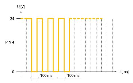
Information about the status of the LUB-S and about the past motor run must be evaluated via an evaluation of the number of edge changes of the output signal. For the evaluation of the edge changes, the rising edge (change of the output voltage at PIN 4 of the LUB-S from a low level (0 V) to a high level (+24 V DC)) must always be counted. The counted number of edge changes corresponds to a one-to-one state of the LUB-S.
