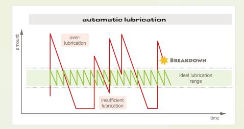
Manual lubrication is inconvinient due to a large variety of different lubricants and applications. Extreme operating conditions such as high temperature, vibrations, shock loads, high loads and contaminants demand frequent and reliable lubrication in order to prevent costly downtime.
