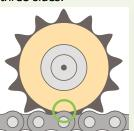
The rollers of the lubrication pinions and lubricating rolls made of open-cell PU foam transfer the lubricant punctually to the surface of the link plates and ensure efficient lubrication. The contact pressure can be optimised by mounting with spring plates.
