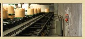
As a battery-operated oil lubrication system, G-LUBE EM B OIL is self-sufficient and therefore particularly flexible. With up to 10 bar delivery pressure, lubrication is possible over longer distances.
