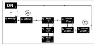
If you would like to change the operating mode, select the Settings menu and move the activation and programming key back to the action area when Mode is displayed.
