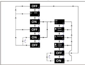
The graphic above illustrates the unchangeable basic flowchart of the LUB-S-V menu navigation as well as the options for branching to submenus.
