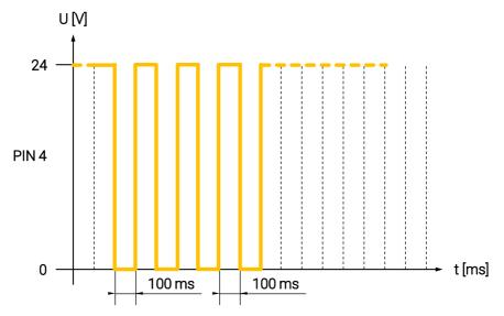
The following graphic shows an example of an output signal.
