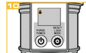
After a short time, the device switches to sleep mode. Only the is shown on the display.
