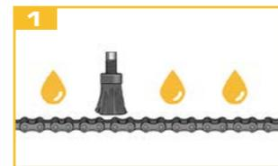
Ensure that a thorough pre-lubrication of the application is carried out before activating the lubricator.
