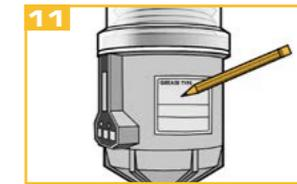
Note the installation and due date on the drive unit.
