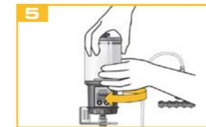
Fix the lubricator in the desired position.
