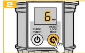
Reset the device after refilling (see „5.6 Reset“) and then set the dispensing quantity again.
