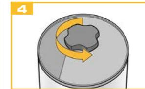
Turn the knob 1-2 turns counterclockwise before closing the cover and do not change the position again during operation.
