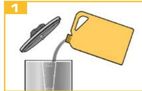
Remove the lid of the oil reservoir and fill it up to the 480 ml level with oil.
