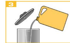
Remove the lid of the oil reservoir and fill it up to the 480 ml level with oil.
