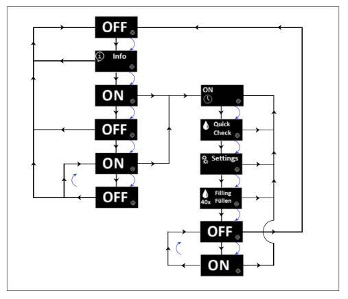
The graphic above illustrates the unchangeable basic flowchart of the LUB-S menu navigation as well as the options for branching to the Sub-menus. The illustration for the operating mode "Setting lubrication cycle duration" was selected as an example.
