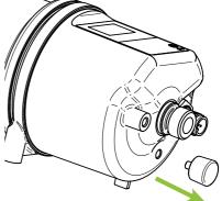
() The activation and programming key is permanently held magnetically in the hole on the underside of the LUB-S.
