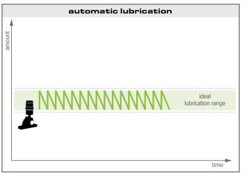
Automatic lubrication systems prevent under- and over-lubrication, thus enhancing the service life of your machines.
