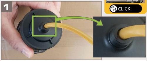
Insert a hose (maximum outer diameter = 6 mm) into the opening at the bottom of G-LUBE and push it as far as possible. A thicker hose would not allow the air to escape during the filling process.
