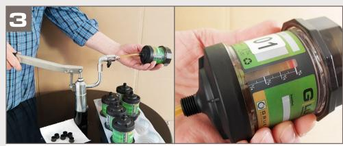
While filling G-LUBE, rotate the device around its own axis to to allow the lubricant to spread evenly. The number of strokes depend on the lubricant and the size of the unit. As soon as you sense a slight backpressure the device is filled completely.
