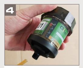
Remove the hose carefully and clean the outlet. Now the device may be screwed on to the lubrication point.
