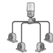
**Multiple point installation** is possible using a progressive distributor. Do not block any connections to the progressive distributor. Instead use a suitable distributor in accordance with the number of lubrication points. Keep the distance between the distributor and the lubrication unit as short as possible.
