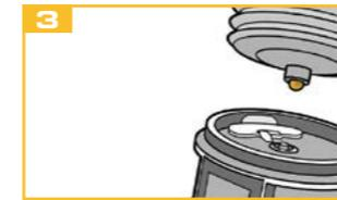
Press the cartridge lightly so that some lubricant escapes.
