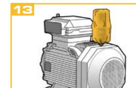
Pull the dust protection cover over the lubricator where necessary.
