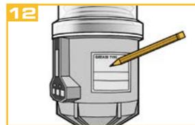
Note the installation and due date on the drive unit.
