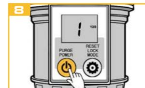
Keep pressed for 5 seconds to switch on the device.
