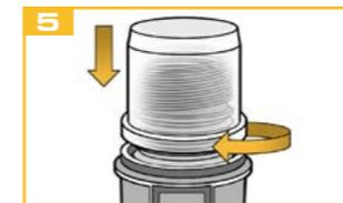
Screw the top section onto the drive unit. The top section locks into place with an audible click.
