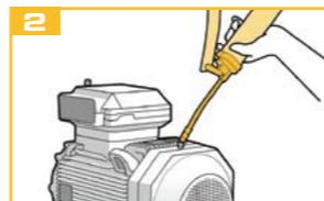
Ensure a clear passage using a manual grease gun.
