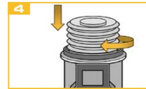
Screw in the cartridge without overtightening it.
