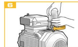
Fix the lubricator in the desired position.
