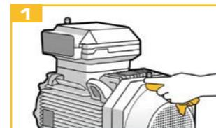
Remove any contaminants around the lube point.
